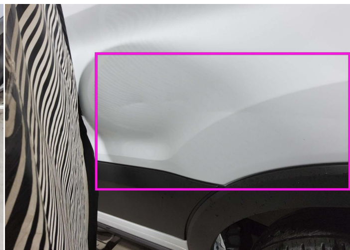
2. Fender / Back - Left Bodywork / Dent / Dent -
