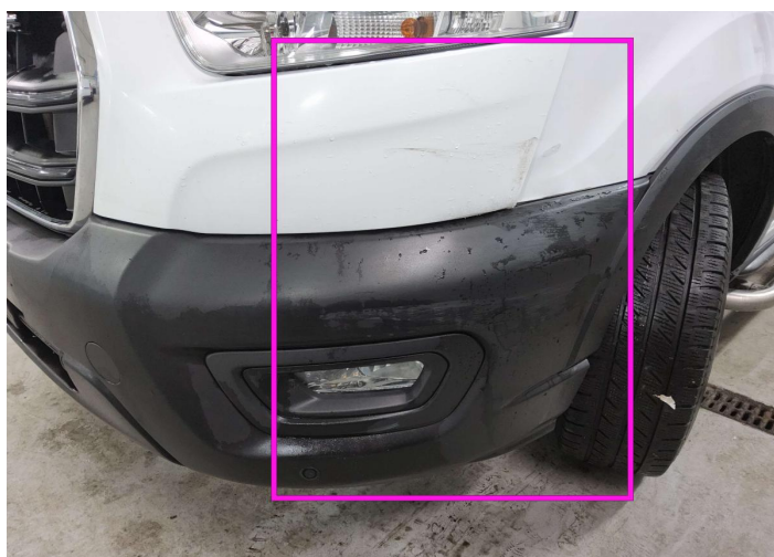
3. Kofanger / front Bodywork / Dent / Deformation -
