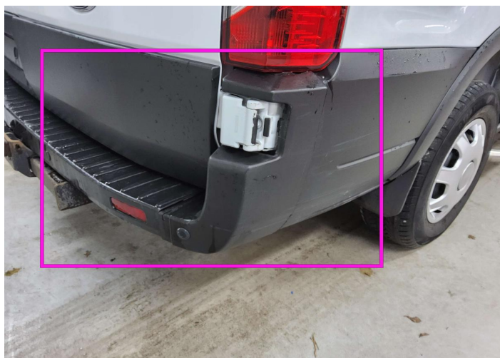
1. Bumper / Back Bodywork / Dent / Deformation -
