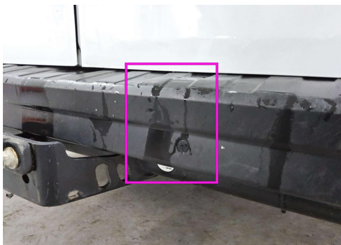
3. Bumper / Back Bodywork / Dent / Deformation -
