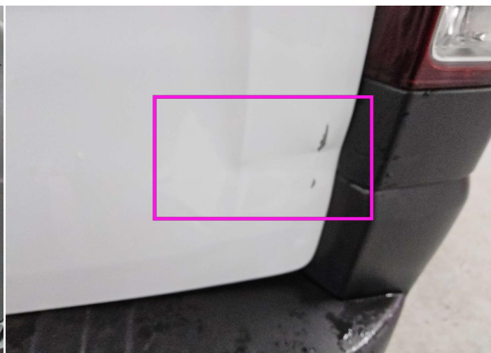
2. Swing Door / Back - Left Bodywork / Dent / Dent -
