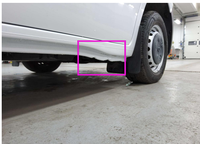
3. Rocker Panel / Center - Right Bodywork / Dent / Deformation -
