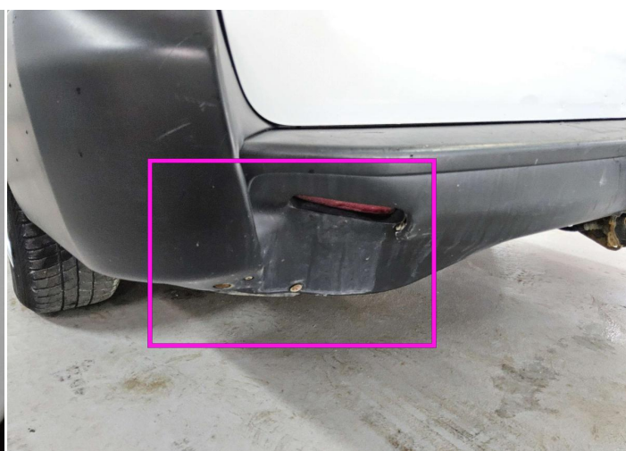
6. Bumper / Back Bodywork / Dent / Deformation -
