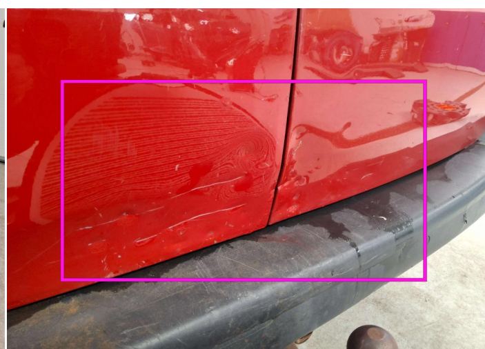
4. Swing Door / Back - Left Bodywork / Dent / Dent -
