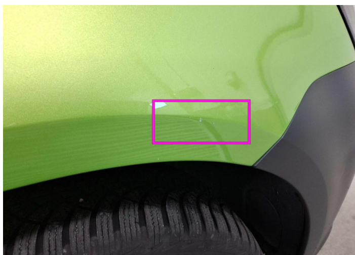
7. Fender / Front - Right Maling / chipping -
